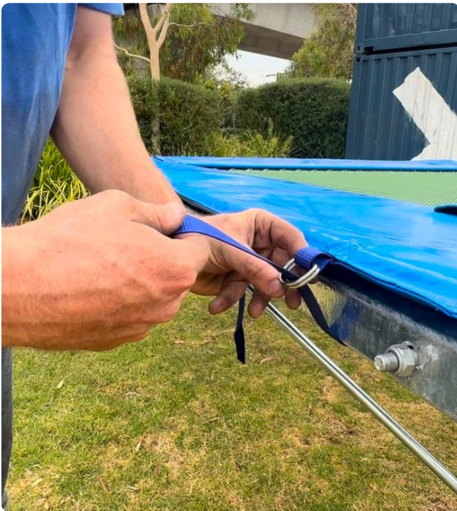
Threading the webbing through the D-ring buckle and pulling it tight.
