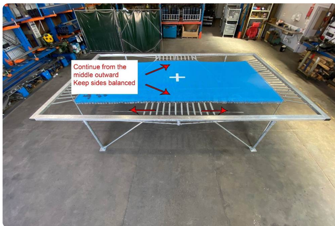
Continue from the middle outward on both sides. Keep the sides balanced.
