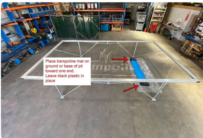
Mat placed inside the frame towards one end, still on its black plastic.
