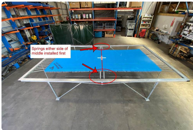
On each long side the first two springs go either side of the middle mark.
