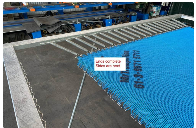
Close-up of a finished end — every clip sprung, ready for the sides.
