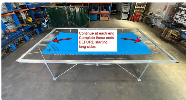
Continue at each end. Complete both ends before starting the long sides.
