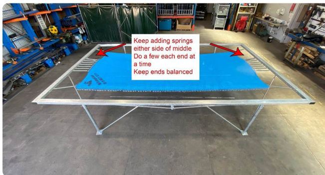
A few springs at each end at a time — keep the ends balanced.
